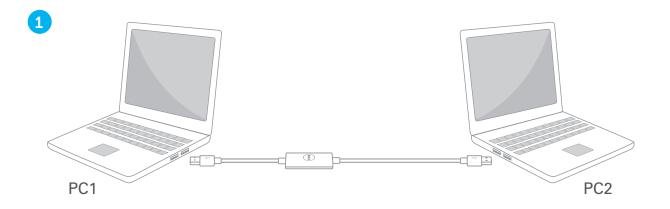
Plug either end of the USB Transfer Cable into PC 1 and the other end into PC 2.
